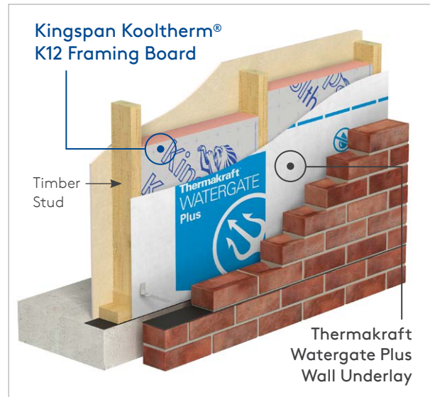
Figure 4. Timber Frame Construction with Insulation between Studs.
