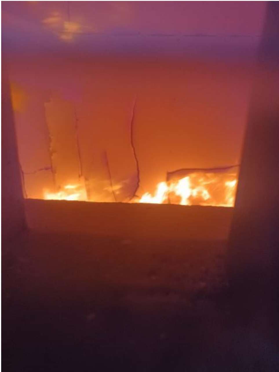
Photograph 9 - View of the exposed side at 17 minutes. Note the flaming and increased size of the cracks
