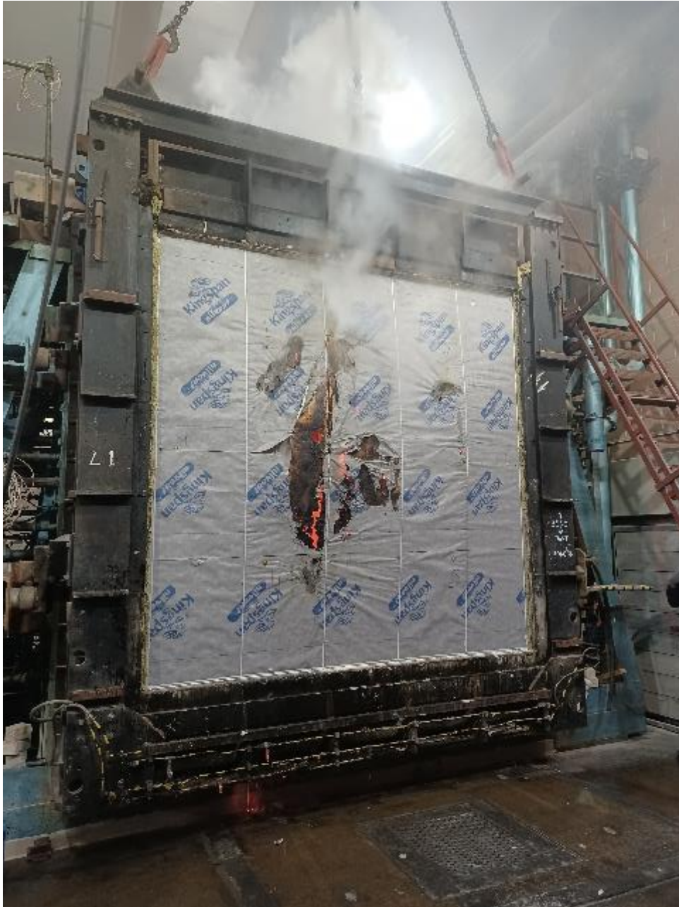
Photograph 12 - View of the unexposed side of the sample after the test.
