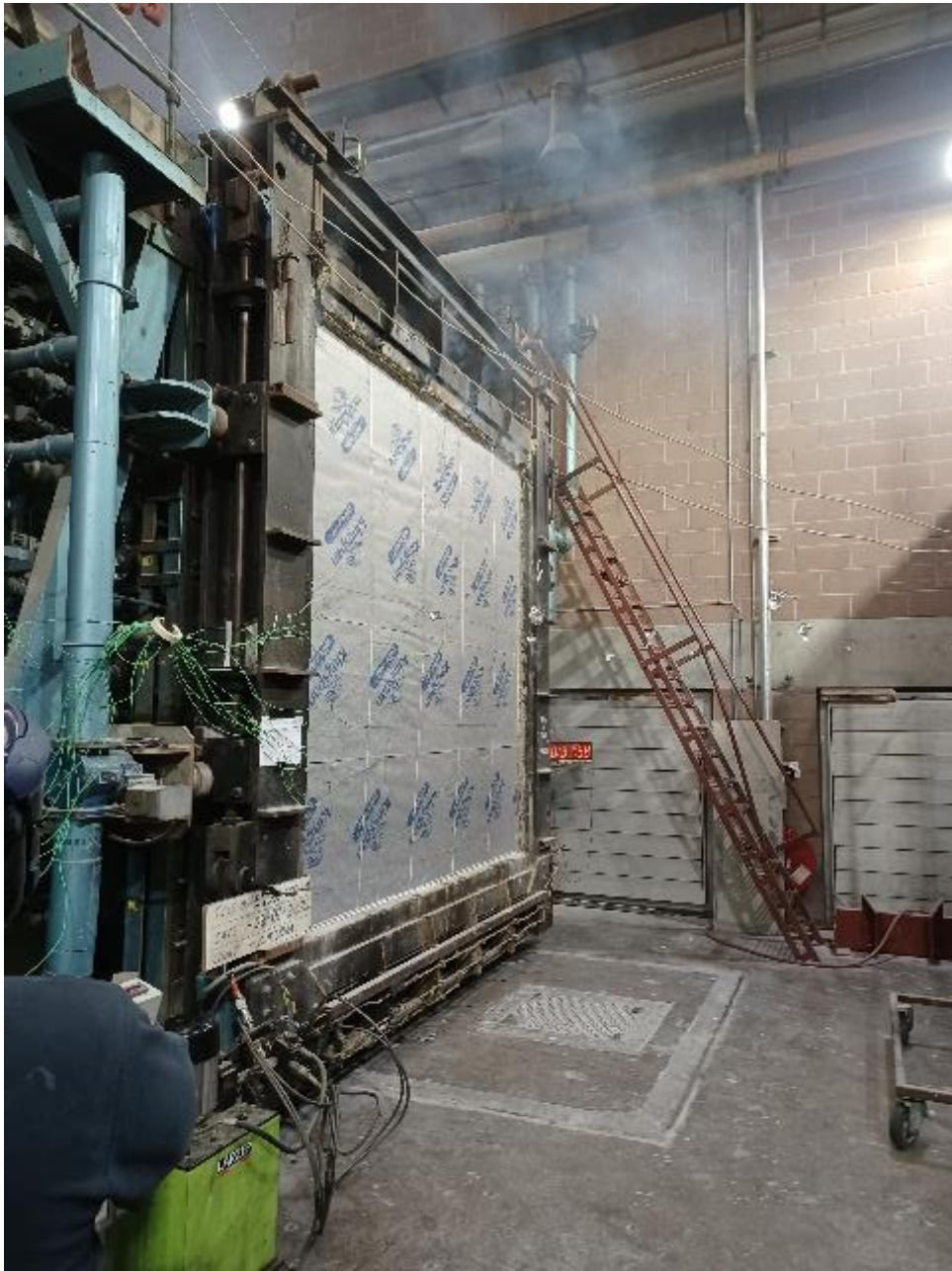
Photograph 11 - View of the unexposed side at 37 minutes. Note the visible deflection.
