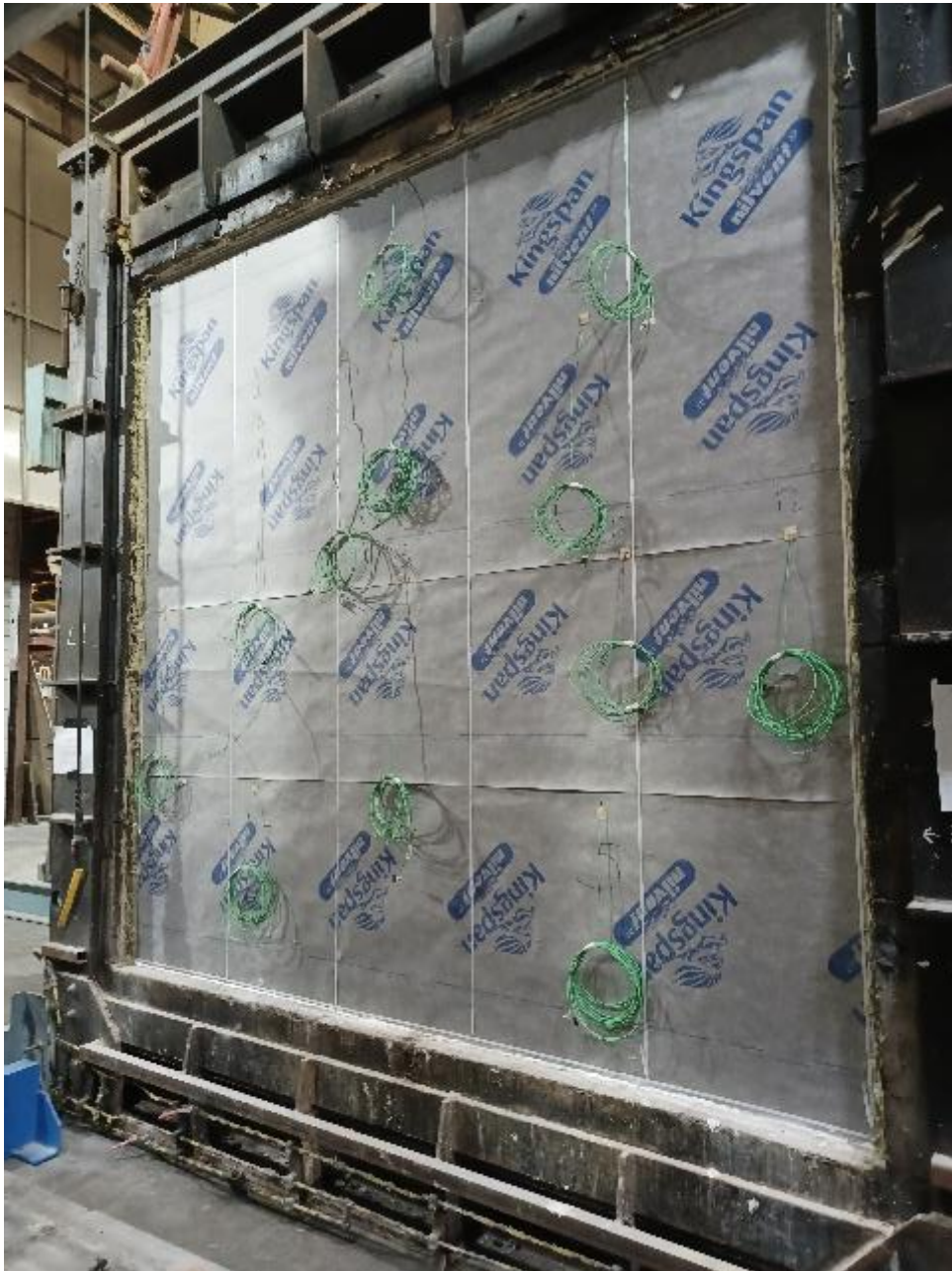
Photograph 7 – View of the unexposed side of the sample prior to the test
