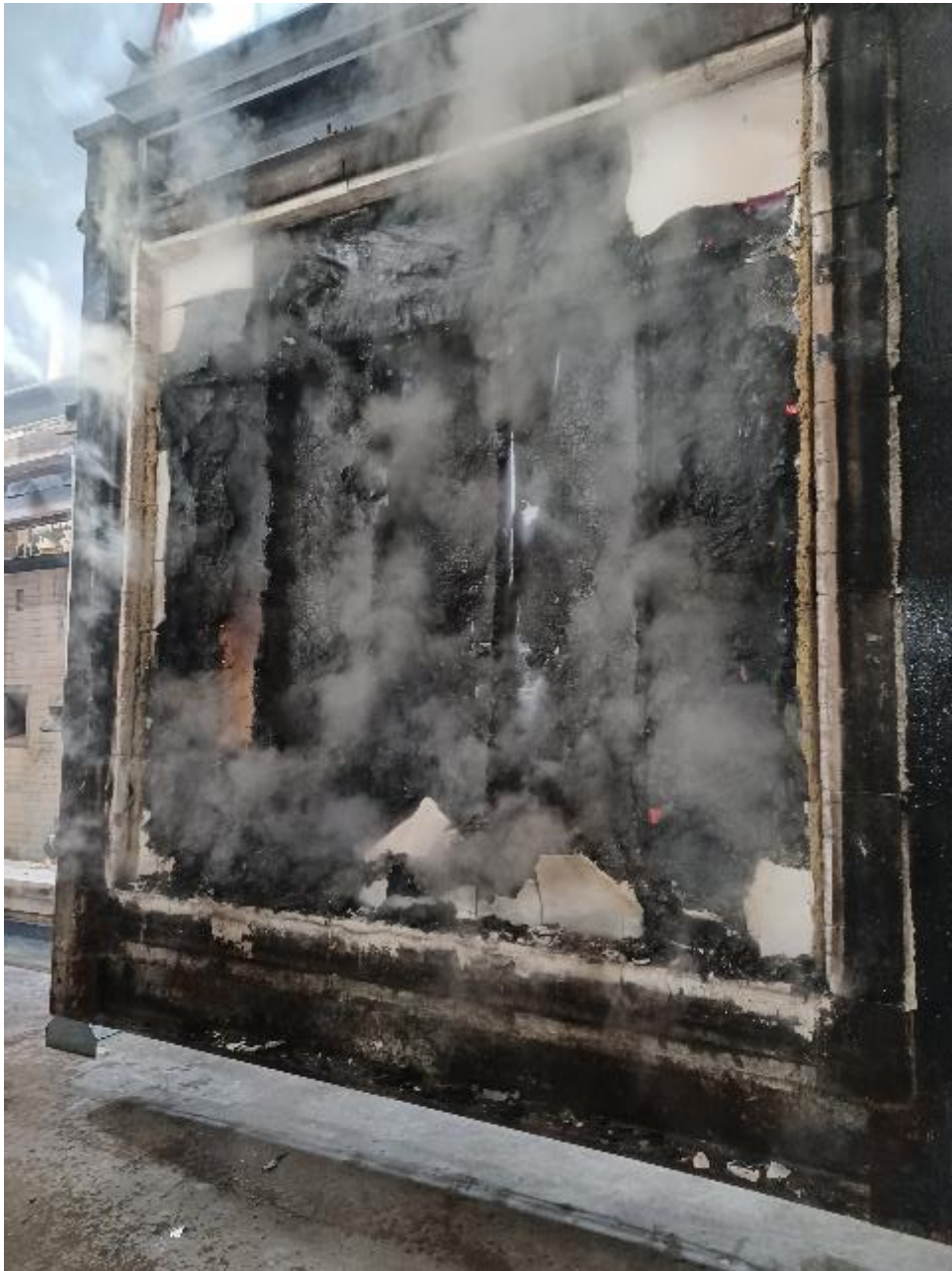
Photograph 13 - View of the exposed side of the sample after the test.
