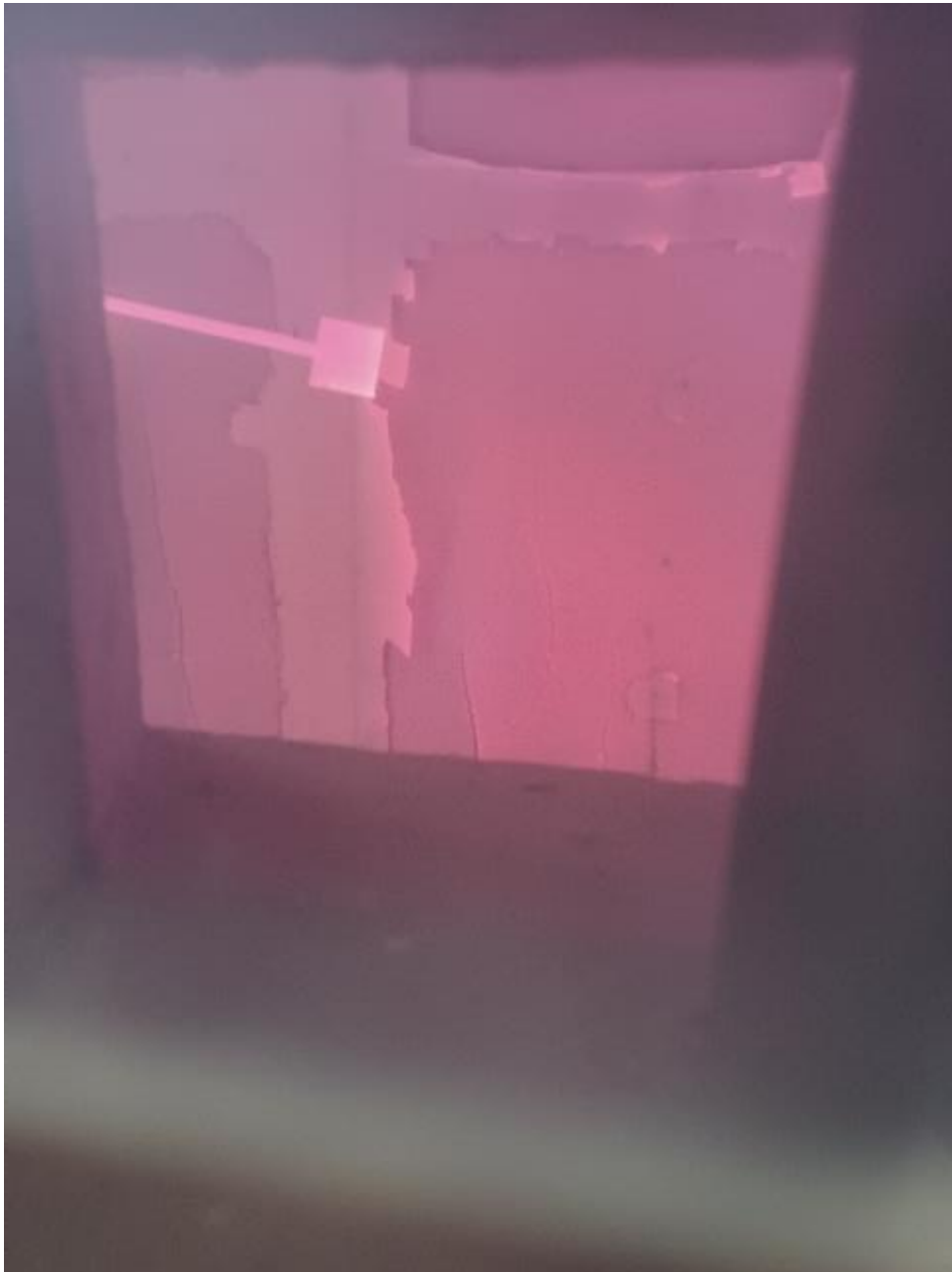
Photograph 8 - View of the exposed side at 11 minutes. Note the vertical cracks forming
