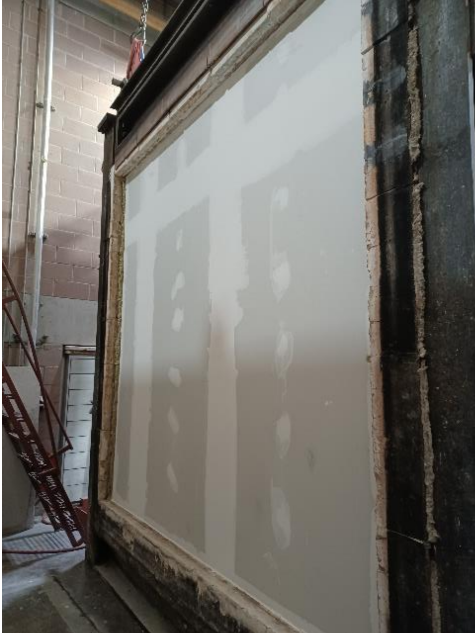
Photograph 6 – view of the exposed side of the sample prior to the test
