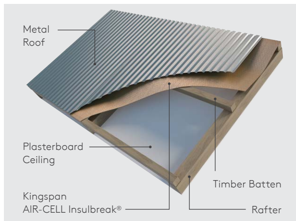
Figure 10. Kingspan AIR-CELL Insulbreak® 55 in a timber framed metal roof sheet, with a raked ceiling.
